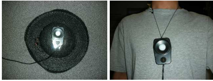
Fig. 5. Left: light sensor on a hat. Right: light sensor as a pendant
