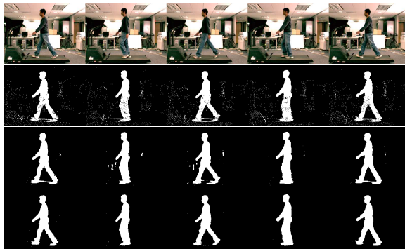
Fig. 3. From top to bottom: (1) Input sequence; (2) Segmentation results using only low-level information; (3) Results after imposing spatio-temporal constraints; (4) Final results after incorporating shape prior.
